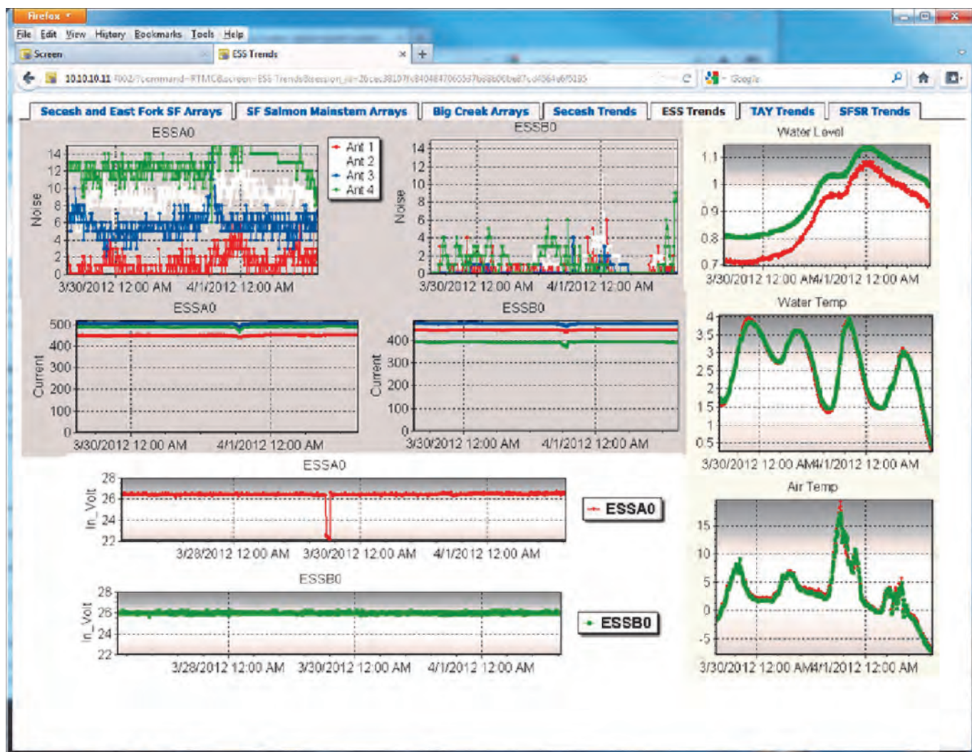
Figure 80. Example of specific instream PIT tag detection site environmental conditions, equipment functions and diagnostic data, and input power levels for the East Fork South Fork Salmon River detection site.
