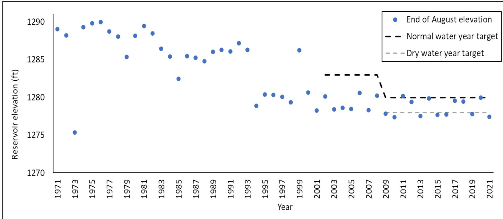
Reservoir elevation (ft; blue dots) at the end of August relative to draft limit (black dash), at Lake Roosevelt, Grand Coulee Dam, 1971 - 2021.
